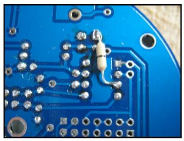
Back side view of completed SA612 ground mod
