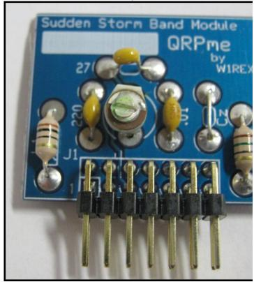
View of completed 40m band module board
