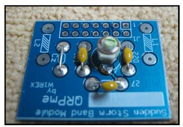
Band module board with caps installed.
