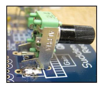
If you purchased the Sudden Storm Soup-up kit, you will want to install those pots instead of the regular pots supplied. The larger Soup-UP pots are designed for vertical mounting, so the mounting leads need to be straightened. The pots are mounted into the larger pot holes. Two cut off component leads can be soldered between the mounting tabs on the pots and a set of extra holes on the pcb pads to provide extra stabilization to the pots.
