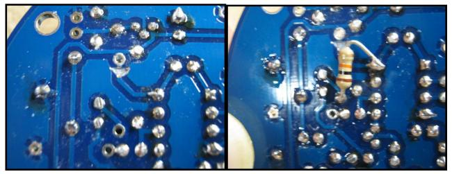
I solate the top pad for R4 then mount R4 to lower pad and IC pin.
