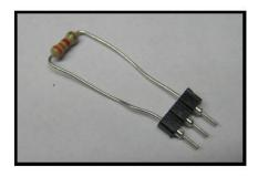
Crystal socket with resistor 'handle'
